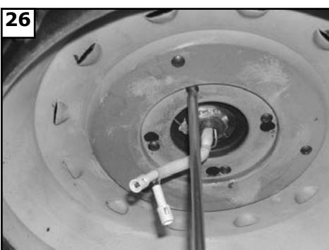
Take plate and place over the 3 screws with key slots and twist to hold in place. Replace the screw removed and tighten all 4 screws securely holding the plate.
